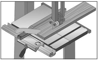
Figure 52. Example of a ripping operation.
